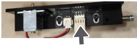
2. Insert the magnetic lock into the printer (picture below) and secure the cable to the metal frame. Connect the cable's end to the top of the printer.
