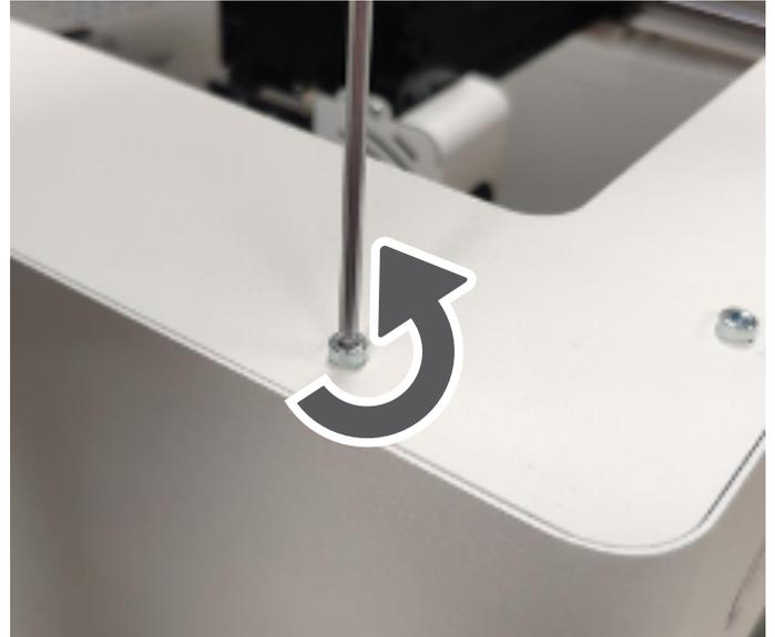
2. Unscrew the back of the dome using the longer screws (Screws are included with the dome ). Then connect the dome fan on the back plate of the printer.
